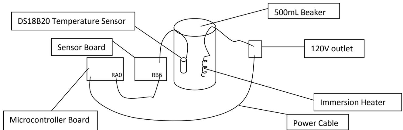
Set up the apparatus as shown in the figure above. Leave the immersion heater unplugged until instructed later. Note, that the temperature sensor attaches to the temperature module, then the RB6 pin on the sensor board is attached to the RA0 pin on the microcontroller board for direct monitoring.
