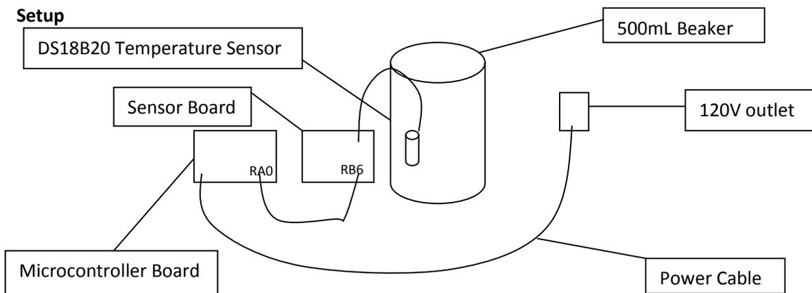
Set up the apparatus as shown in the figure above. Note, that the temperature sensor attaches to the temperature module, then the RB6 pin on the sensor board is attached to the RA0 pin on the microcontroller board for direct monitoring.
